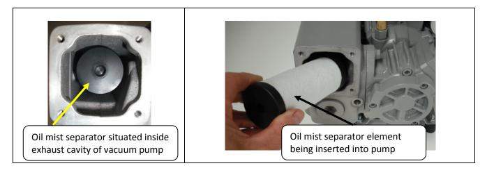
The oil mist separator cavity is normally closed off by a cover plate. If not already fitted, we recommend fitting an elbow into the exhaust port of the pump and facing it downwards. This will reduce the likelihood of dust entry to the pump when it is stopped or running at high vacuum (= very low air flow)
