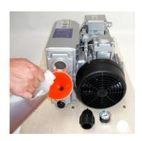
DO NOT OVER FILL. Fill to between the MIN and MAX marks.
