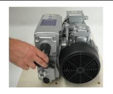
Unscrew the back pressure gauge/oil filler cap. This should also be hand tight and removable by turning the gauge case anti-clockwise. If tight, apply a 30 mm (1 3/16") AF spanner to the oil filler cap the gauge is attached to.
