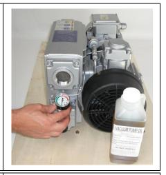
Replace the exhaust elbow. Screw in hand tight only and point the opening downwards at about  $45^{\circ}$ . Angling the exhaust downwards will reduce dust entry into the pump when it is stopped or running at high vacuum (when there is no air flow).
