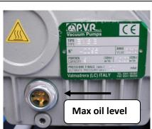
DO NOT OVERFILL! Fill to a maximum of ¾ level on the sight glass.
