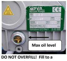
DO NOT OVERFILL! Fill to a maximum of ¾ level on the sight glass.
