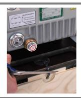
Lift the machine off the plywood base. Leave the castor brakes locked until assembly has been completed.
