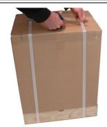
Lift the complete carton off the plywood base to expose the cart and vacuum pump.
