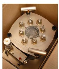
Lift the resin trap out of the carton using the handles.
