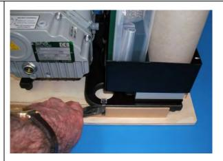
Lock the castors when removing the machine from docking station
