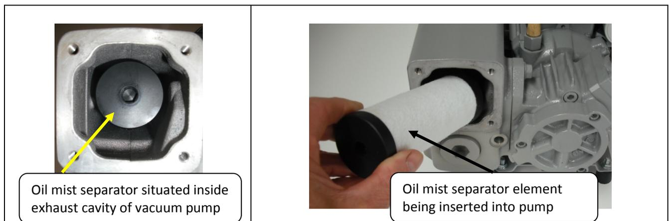
Oil mist separator situated inside exhaust cavity of vacuum pump
