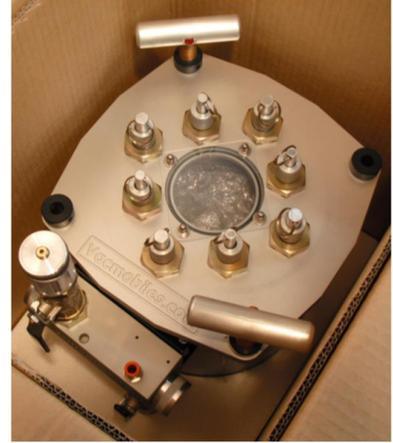
Lift the resin trap out of the carton using the handles.
