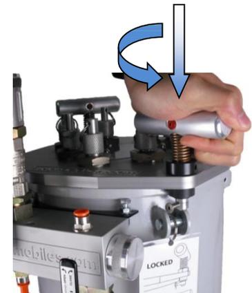
Complete assembly and prepare for operation as described in the instruction manual supplied with the machine, with the two key steps being adding oil to the vacuum pump and making sure there is a catchpot in the resin trap. See below.
