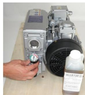
Fit a small funnel to the oil fill port and add the correct grade of vacuum pump oil.
