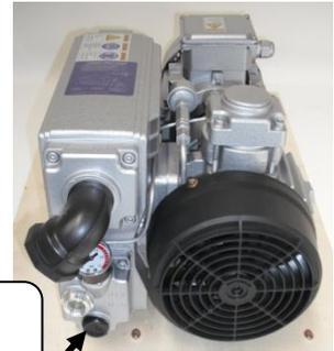
The external oil filter should be replaced at every oil change. As some oil will drip when the oil filter is removed, place a suitable collection tray under the oil filter.
