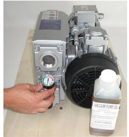
Replace the exhaust elbow. Screw in hand tight only and point the opening downwards at about 45°. Angling the exhaust downwards will reduce dust entry into the pump when it is stopped or running at high vacuum (when there is no air flow).
