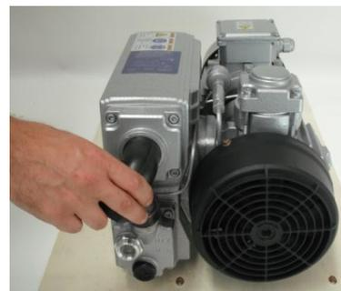
Unscrew the back pressure gauge/oil filler cap. This should also be hand tight and removable by turning the gauge case anti-clockwise. If tight, apply a 30 mm (1 3/16") AF spanner to the oil filler cap the gauge is attached to.
