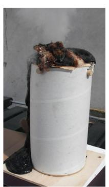
Let's look at our simplified infusion set-up again – this time with the resin catchpot in danger of overflowing.
