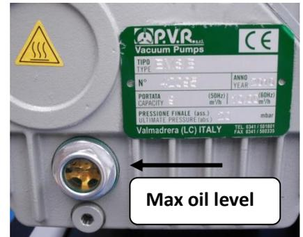
**DO NOT OVERFILL! Fill to a maximum of  $\frac{3}{4}$  level on the sight glass.**
