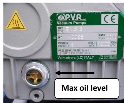
**DO NOT OVERFILL! Fill to a maximum of  $\frac{3}{4}$  level on the sight glass.**
