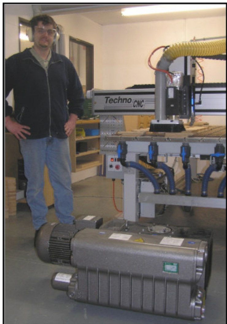
Above, CNC technician Roger Farmer prepares to connect a new VABS supplied PVR 300 m 3 /hr 5.5kW vacuum pump to the Techno LC+4896 at Waka.
