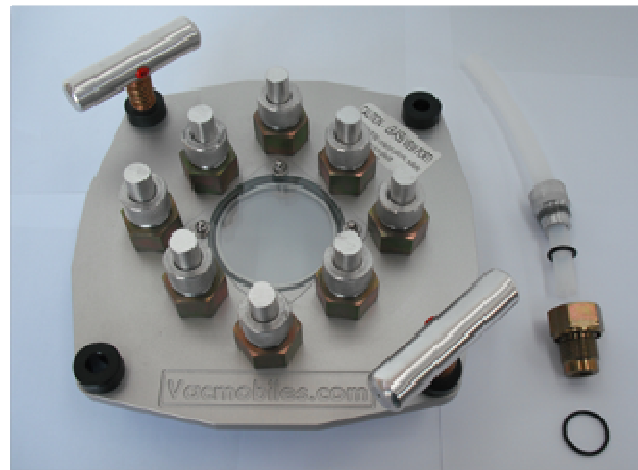
Machined aluminium lid with up to 8 O-ring sealed tubing glands and 75 mm (3”) glass view-port (protected on both sides with disposable clear PVC shields). Easy-to-use “Twist-Lock” handles built into lid.
