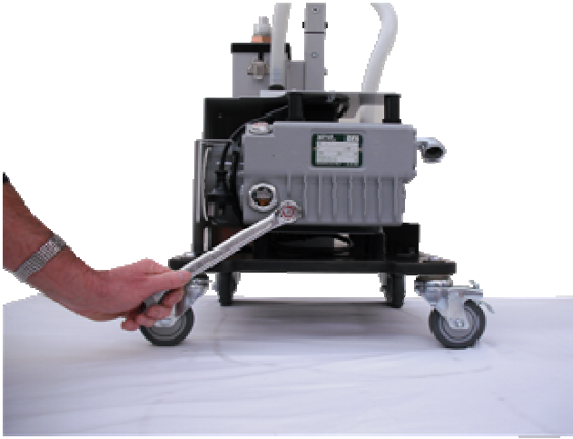
For PVR pump use 22 mm (7/8") AF wrench
