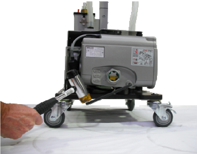
For Becker pump use 8 mm (5/16") Allen Wrench. To loosen, hit down sharply, as shown
