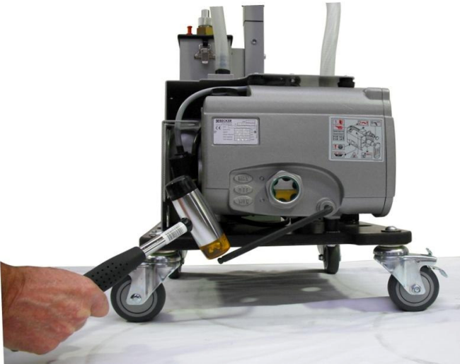
For Becker pump use 8 mm (5/16") Allen Wrench.
