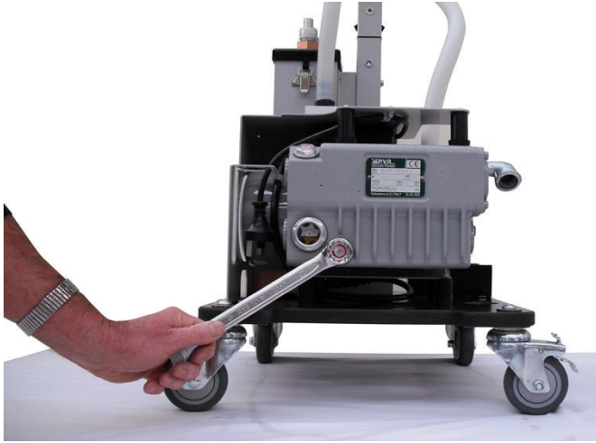
For PVR pump use 22 mm (7/8") AF wrench
