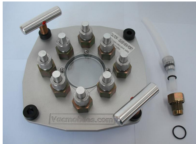
Machined aluminium lid with up to 8 O-ring sealed tubing glands and 75 mm (3") glass view-port (protected on both sides with disposable clear PVC shields). Easy-to-use "Twist-Lock" handles built into lid.
