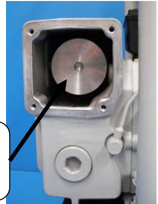
Exhaust oil mist filter (typical)
