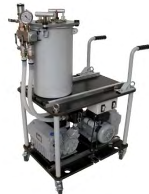
2 pumps and 1 resin trap
