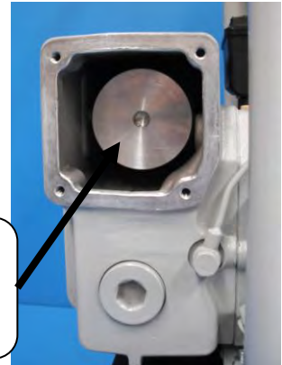
Exhaust oil mist filter (typical)
