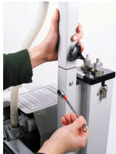
2. Unscrew top fixing bolt
