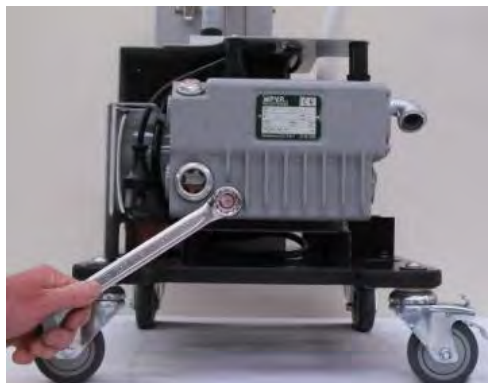
Oil drain on PVR EM20 pump
