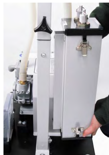
3. Lift resin trap upwards
