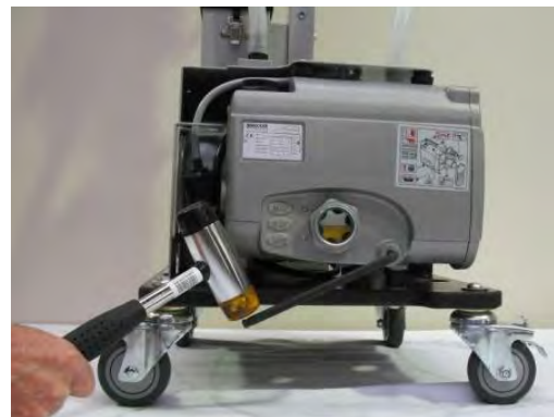
Oil drain on Becker U4.20 pump
