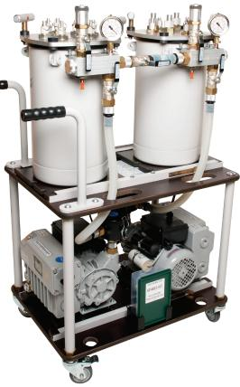
Machines with 2 vacuum pumps, 2 resin traps and the optional interconnect valve (as pictured) allow instantaneous changeover from single vacuum level use to dual vacuum level use.
