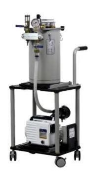
Although we recommend having access to at least 2 vacuum systems when infusing large and high value composites, a single Modular 2S machine will comfortably infuse laminates up to 100 m² (1,100 ft²) and larger, as long as the resin overflow from the laminate can be limited to 12 litres (3.1 US gallons). For information on controlling the resin overflow from infused laminates, please see our website note "Peel ply resin breaks" (http://www.vacmobiles.com/peel\_ply\_resin\_breaks.html).
